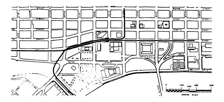
FIGURE 5 ALTERNATIVE E FOUR-GUIDEWAY CENTRAL SECTION ON BAY STREET Each line represents a dual guideway only Central Station is shown
